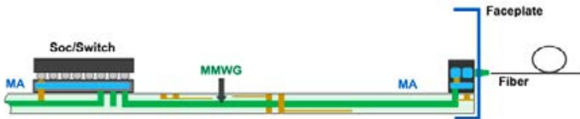
FIGURE 3B - Proposed Interconnection Scheme for Chip to Module (Chip) : CPO-like
