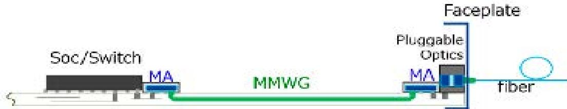
FIGURE 3A - Proposed Interconnection Scheme for Chip to Module (Chip) : NPO-like
