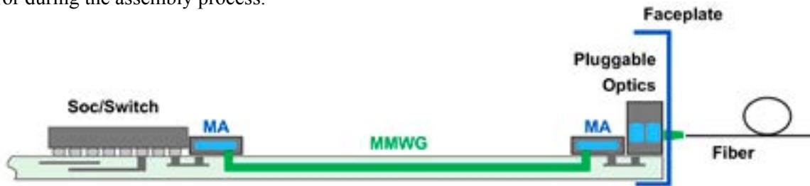
FIGURE 3A - Proposed Interconnection Scheme for Chip to Module (Chip) : NPO-like
