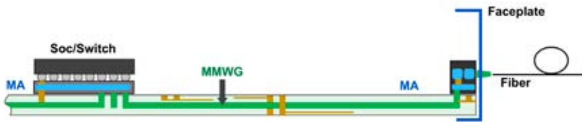
FIGURE 3B - Proposed Interconnection Scheme for Chip to Module (Chip) : CPO-like
