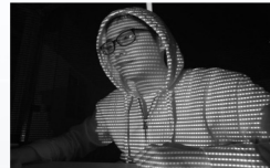
Flash solid-state: VCSELs + SPADs [Credit: Ouster]
